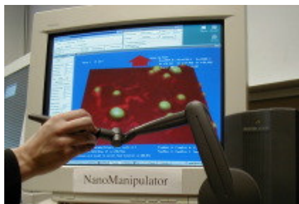
Figure 1. Commercialized version of the nanoManipulator interactive graphics + haptic interface to AFM.
