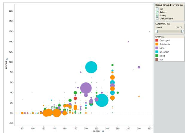
Figure 1. Kinetic energy of bird strikes in the flight envelope. Size represents amount of kinetic energy, color indicates damage to the plane.
